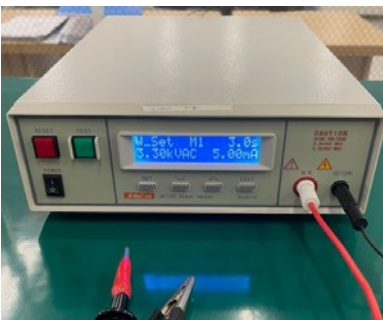
■ High voltage test
